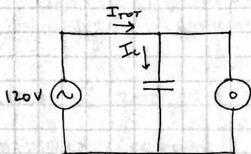
$$\begin{aligned}\bar{V} &= 120V \angle 0^\circ \\ \bar{I}_L &= 8A \angle -75^\circ \\ &= 2 - j 7.75 A\end{aligned}$$
