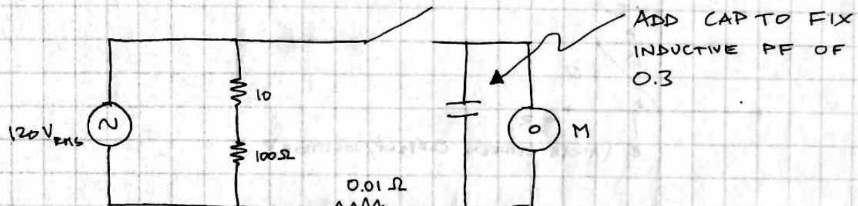
$$V = 120V \angle 0^\circ \quad I = \frac{11.2A}{\sqrt{2}} = 8A_{\text{RMS}}$$
