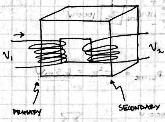
IRON IN CHANNELS MAGNETIC FLUX
