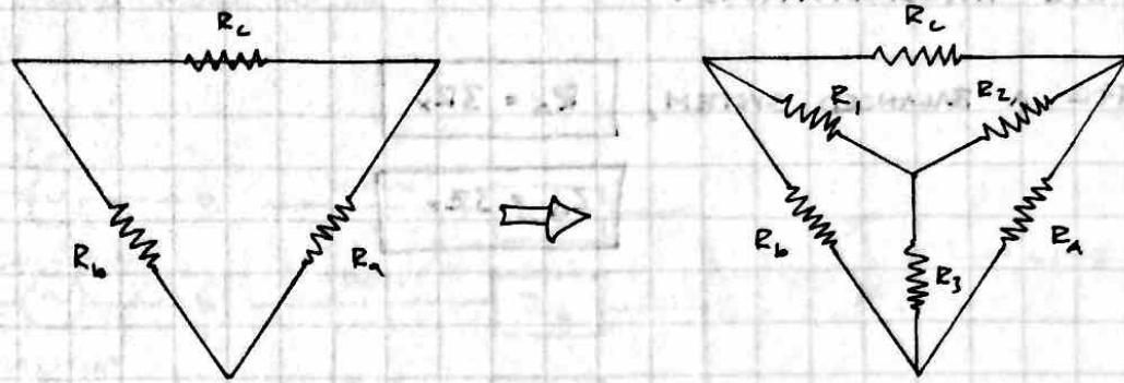
EACH RESISTOR IN THE WYE NETWORK IS THE PRODUCT OF THE TWO ADJACENT  $\Delta$  BRANCHES, DIVIDES BY THE SUM OF THE THREE  $\Delta$  RESISTORS
