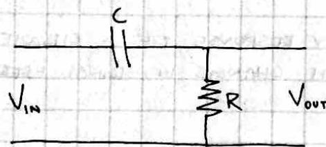
$$H(j\omega) = \frac{V_{out}(j\omega)}{V_{in}(j\omega)} = \frac{R}{R + j\omega RC} = \frac{j\omega RC}{1 + j\omega RC}$$
