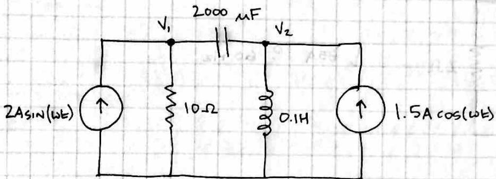
LOOKING FOR VOLTAGE @  $V_1, V_2$
