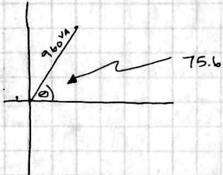
$$\begin{aligned}P &= 239 \text{ W} \\ Q &= 930 \text{ VAR}\end{aligned}$$
