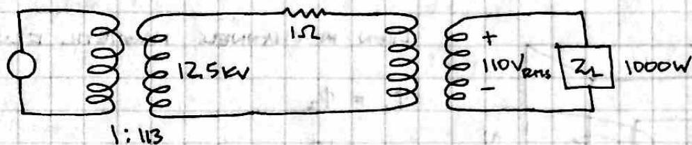
$$I_{\text{LINE}} = \frac{9.1A}{113} = 80mA, P_{\text{LINE}} = I^2 R = \underline{6.5mW}$$
