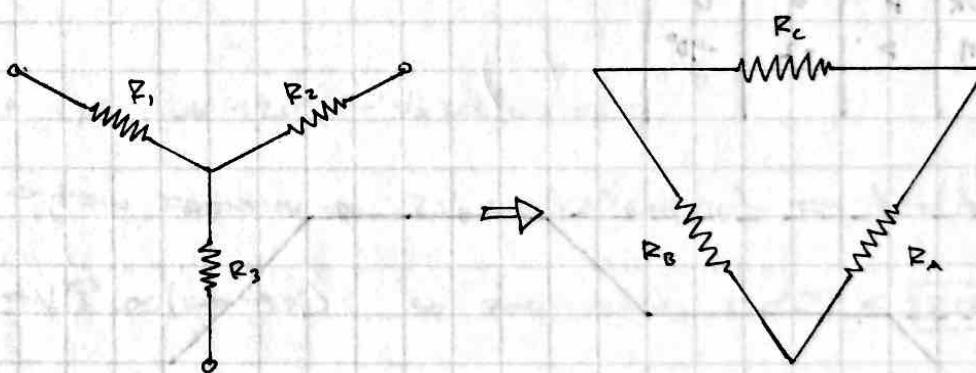
EACH RESISTOR IN THE DELTA NETWORK IS THE PRODUCT OF ALL POSSIBLE WYE RESISTORS TAKEN TWO AT A TIME, DIVIDED BY THE OPPOSITE Y RESISTOR.
