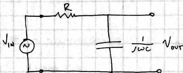
$$\frac{V_{\text{OUT}}}{V_{\text{IN}}} = \frac{1}{R + j\omega C}$$
