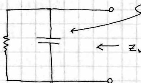
$$Z_N = \frac{(100\Omega)(-j100\Omega)}{(100\Omega) + (-j100\Omega)} = 50 - j50\Omega$$
