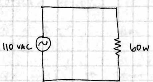
$$P = \frac{(V_{\text{RMS}})^2}{R}$$
