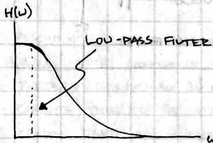
$$|H(\omega)| = \sqrt{\left(\frac{1}{1+j\omega\omega_0}\right)^2 + \left(\frac{1}{1-j\omega\omega_0}\right)^2}$$
